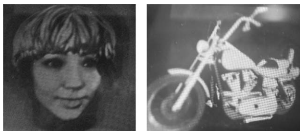
Fig. 9 Reflective/Lippmann parallax true-color holographic stereogram with a real size of 16 cm 2 : left, portrait; right, computer-generated bike.
