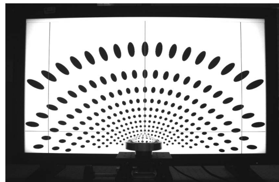
Fig. 4. LCD monitor displaying the flat null screen and test surface.
