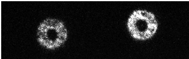
Figure 6. Instantaneous image of the scintillation pattern cast over the analysis plane of LOLAS. The pupils are misaligned by 5^\circ from the EMCCD rows.
