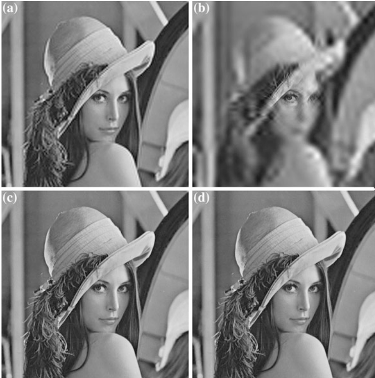
Fig. 55.5 Foveated image with the proposed window and different compression methods. a DCT-based foveated compression, b wavelet-based foveated compression with db9/7 and energy profile quantization, c wavelet-based foveated compression with db9/7 and tukey window scaling quantization, d wavelet-based foveated compression with db9/7 and JPEG Type 1 quantization
