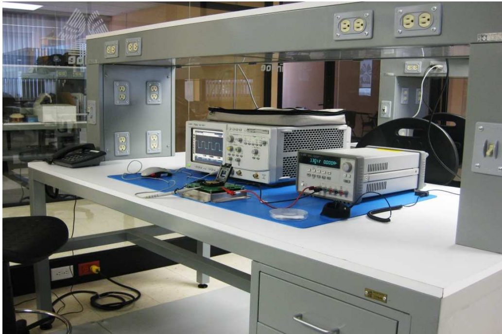
Figure A.4: Test setup for the Off-Chip measurements of the fabricated three-stage ring oscillators.
