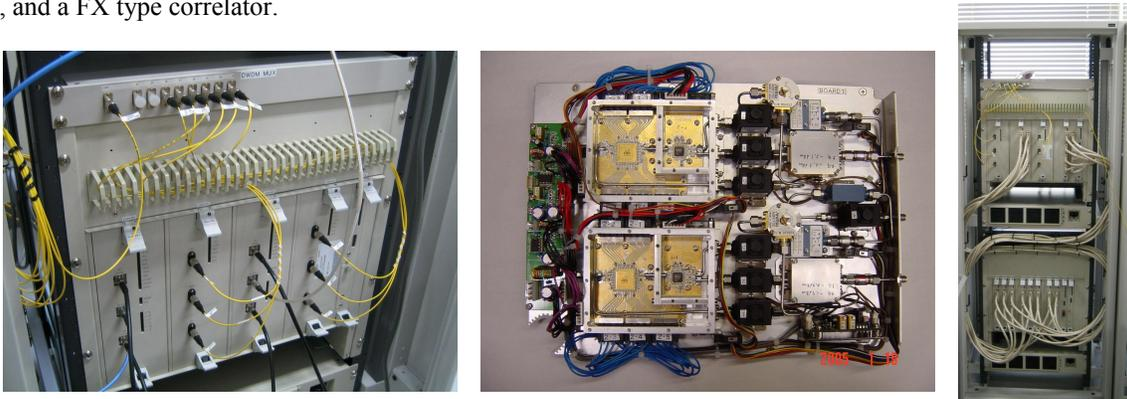
Fig. 7. (left) The “front-end” section of the WHSF system mounted in the receiver cabin, (middle) Close up view of the ADC board, (right) the digital correlator section of the WHSF system.
