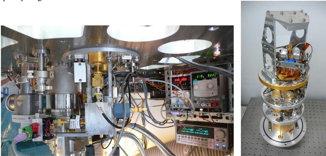
Fig. 6. (left) The CATS345 receiver system mounted on the ceiling of the ASTE receiver cabin. The cryostat employs a plug-in cryogenic system for receiver cartridges. (right) The receiver cartridge of CATS345 in the lab.
