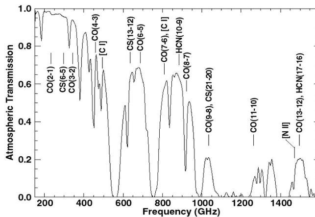
Fig. 2. Atmospheric transmission at the ASTE site (Pampa la Bola) measured by a Fourier-Transform Spectrometer<sup>3</sup>. The figure shows that our site has 60% or more transmission within major atmospheric windows.
