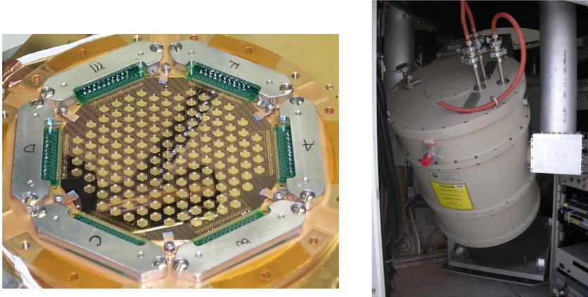
Fig. 4. (left) The AzTEC bolometer array, (right) The AzTEC cryostat mounted in the receiver cabin of ASTE
