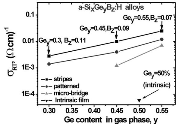
Fig. 4. Conductivity dependence on the Ge gas content,  $Ge_y$ .
