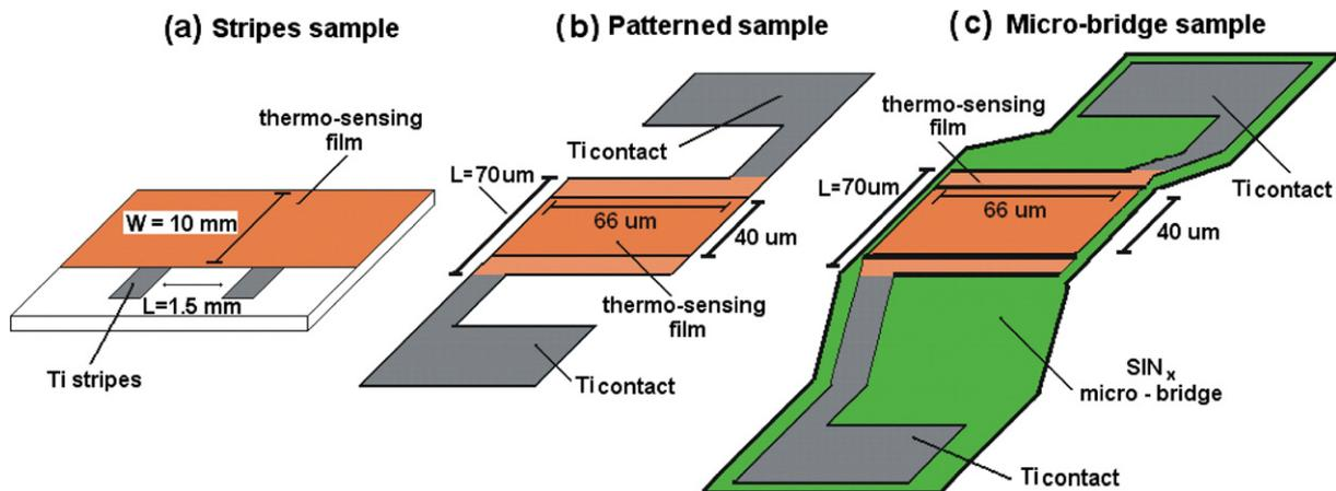
Fig. 1. Three different samples for electrical characterization: (a) stripes, (b) patterned and (c) micro-bridges.
