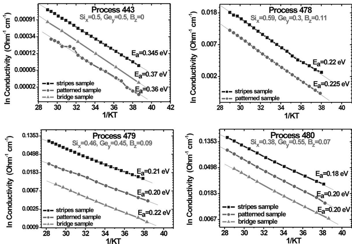
Fig. 2. Conductivity dependence with temperature for the different thermo-sensing films (process: 443, 478, 479 and 480).
