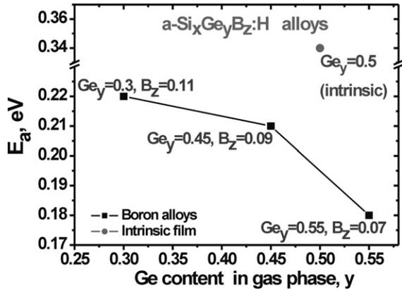
Fig. 3.  $E_a$  as function of Ge gas content,  $Ge_y$ , in the boron alloys,  $a-Si_xGe_yB_z:H$ .
