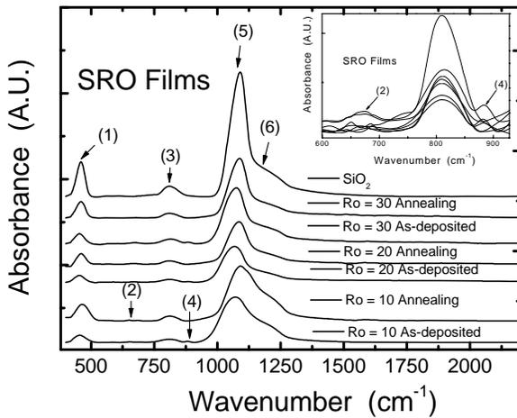
**Figure 2.** FTIR Absorption Spectra of the SRO films of  $Ro = 10, 20$  and  $30$  after different annealing, and absorption spectra of thermal SiO<sub>2</sub>. The capital letters (R), (B) and (S) mean Rocking, Bending and Stretching vibration modes.
