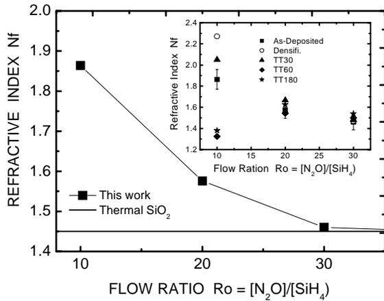
**Figure 1.** Refractive index as a function of  $Ro$  for as-deposited films, a comparison with thermal SiO<sub>2</sub> is done. The inset shows the Refractive index as a function of  $Ro$  for different annealing times.
