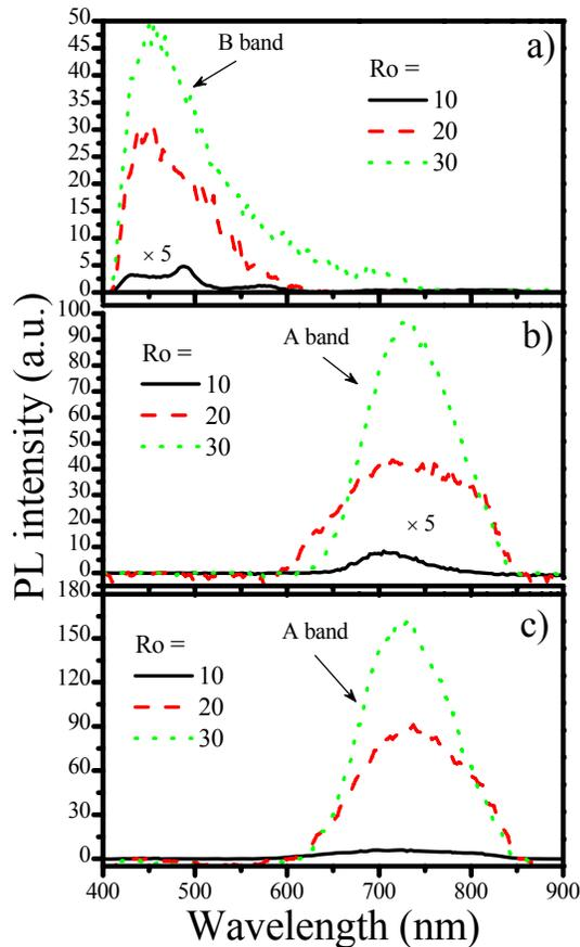
**Figure 4.** PL spectra of SRO with  $R_o = 10, 20$  and  $30$  and a) as-deposited, b) densified at  $1000\text{ }^\circ\text{C}$  for  $30$  min, and c) thermally annealed at  $1100\text{ }^\circ\text{C}$ .
