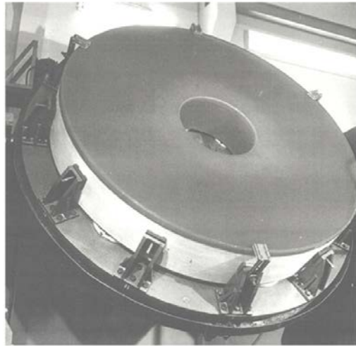
Fig. 6. Grinding and polishing machine constructed at INAOE, and the 210 cm mirror ready to be polished after the central hole was ground.
