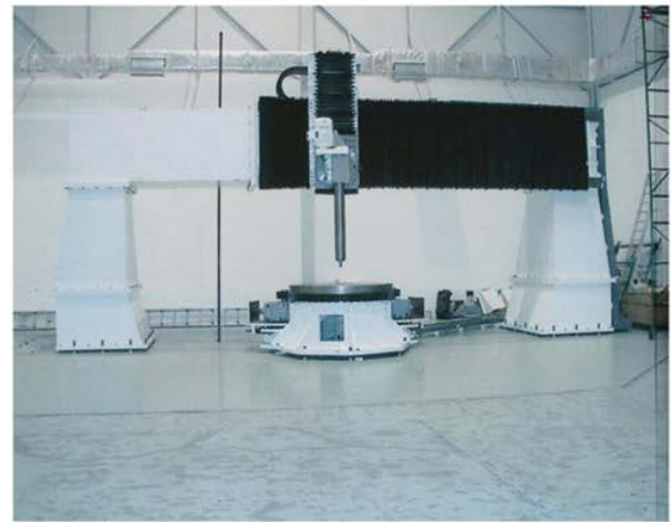
Fig. 10. Measuring XYZ instrument and polishing machine with capacity for mirrors with maximum 8 m in the diameter.
