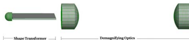
Fig. 9. Design of the shape transformer with the auxiliary demagnifying optics composed of two 3-mm diameter lenses.
