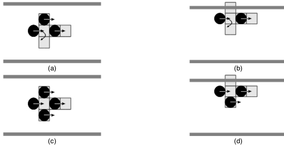
Figure 5. Specific pedestrian and combined encounters synthesized as the binary encounter shown in Figure 4(c). The domain of turn angle and step size are constrained as a pedestrian perceives an obstacle or partners within its perceptual field.
