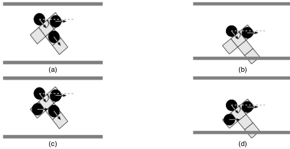
Figure 7. Specific pedestrian and combined encounters synthesized as the binary encounter shown in Figure 6(c). The domain of the step size is constrained as a pedestrian perceives an obstacle or partners within its frontal perceptual field.
