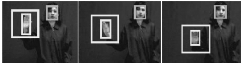
Figure 4. Example of the results of hand tracking through a sequence of 3 images.
