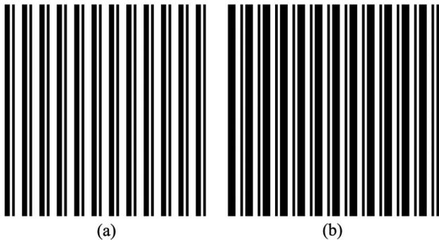
Fig. 10. 7 bit substructured rulings of the Katyl type: (a) positive and (b) negative.
