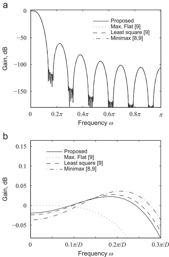
**Fig. 10.** Overall magnitude response of the GCF filter and the compensation filters in the design example.
