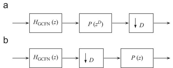
Fig. 2. Decimation block diagrams. (a) Generalized comb filter  $H_{GCFN}(z)$  and compensation filter. (b) Efficient structure for decimation.
