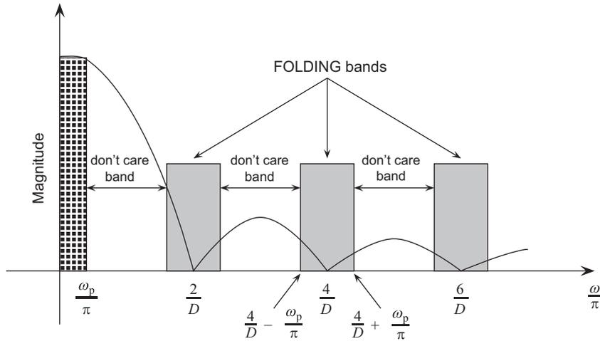
Fig. 1. Magnitude characteristic of the comb filter with decimation factor  $D$ .
