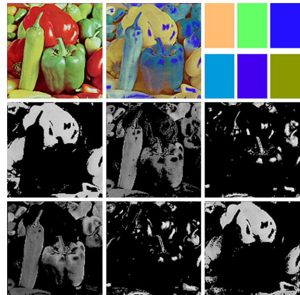
Fig. 5 1st row, left to right: sample RGB color image, transformed HSI color image, saturated colors obtained from \overline{W} (upper horizontal array of colored rectangles) and \overline{M} (lower horizontal array of colored rectangles); 2nd and 3rd rows: grayscale segmented images derived from \overline{w}^j , respectively, \overline{m}^j for j = 1, 2, 3, showing “red/green” pepper regions and bright reflected light regions
