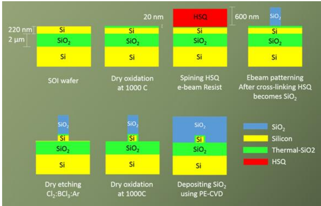
Figure 4.6. Fabrication process flow. (Figure extracted from reference [35] )
