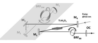
FIG. 2 Dual wavelength laser setup based on a Ti:Al<sub>2</sub>O<sub>3</sub> crystal. M<sub>1</sub> to M<sub>5</sub> are dielectric IR mirrors, M<sub>4</sub> is a dichroic mirror. OC: Output Coupler. M<sub>2</sub> and M<sub>3</sub> form a 90° periscope. BRF<sub>BB</sub> is the narrow broadband filter and BRF<sub>DW</sub> is the thick filter as described in the text.
