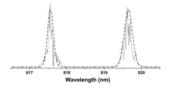
FIG. 4 Ti:Sapphire laser dual wavelength emission (817.57 nm and 819.63 nm) with spectral separation  $\Delta v$  = 0.953 THz.
