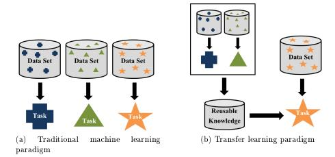
Figure 4.1: Illustration of the differences between the two learning paradigms. Traditional machine learning algorithms (a) build a model from domain specific examples, whereas transfer learning (b) extracts useful knowledge from what has already been learned to build the model for a new task.
