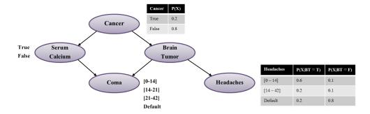
Figure 1.1: An example of a Temporal Nodes Bayesian Network. Each node represents an event, and the arcs (arrows) between them temporal relationships. A probability distribution is associated to every node. For simplicity only the probability tables for "Cancer" and "Brain Tumor" are shown.
