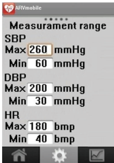
FIGURE 6: Measurement thresholds set on the Android graphic user interface.
