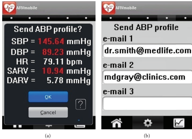
FIGURE 8: The ARVmobile-Blackberry graphic user interface for (a) instantaneous feedback and (b) forwarding an ABP profile to selected recipients.
