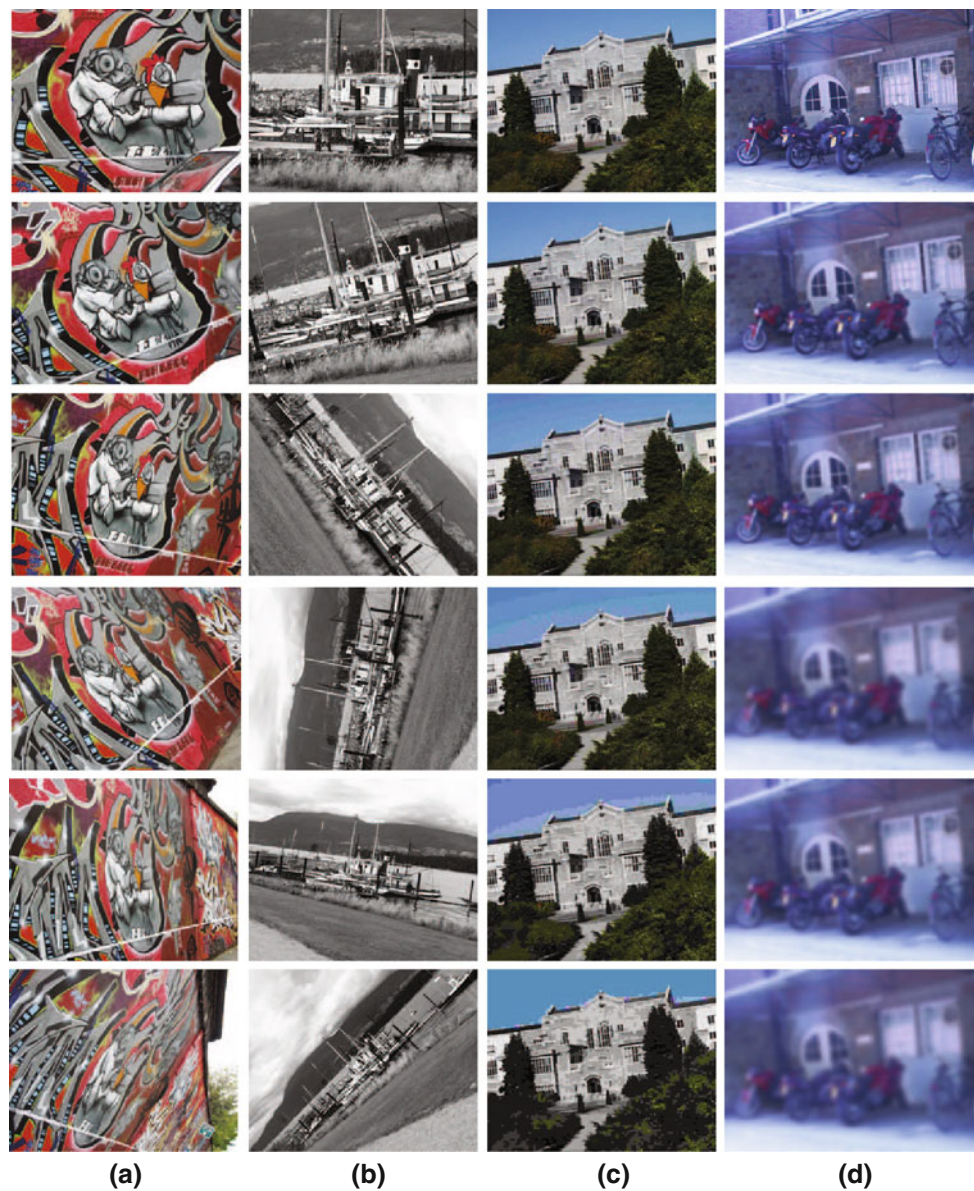
Fig. 15 Test set. In a changes in viewpoint, b changes in scale and rotation, c variations in JPEG compression, and d variations of blur. For each of these subsets the first image is taken as reference image
