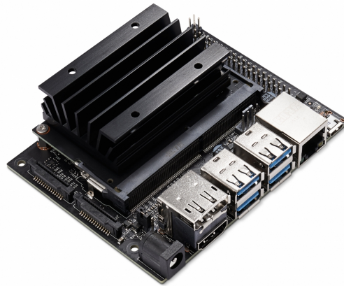
Figure 2.1: Jetson Nano Developer Kit [1]
