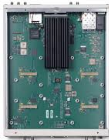
Figura 4.10: Tarjeta madre del USRP X300. Tomado de https://www.ettus.com/all-products/x310-kit/
