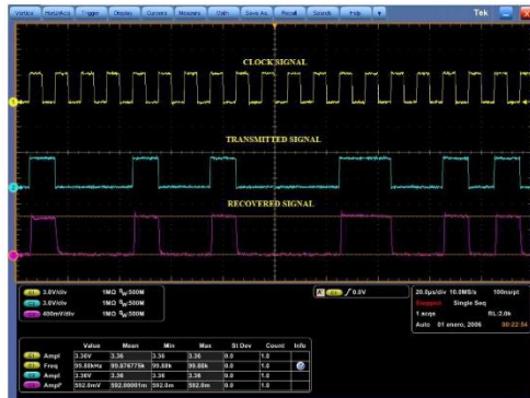
Fig. 6. Screen of the oscilloscope illustrating the traces for the clock, transmitted, and received signals.
