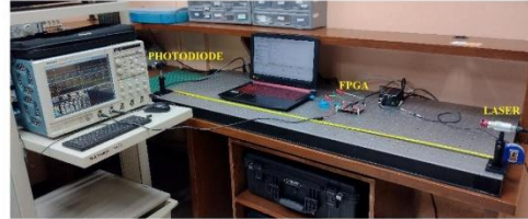
Fig. 7. Photograph of the experimental arrangement FSO indoor prototype.
