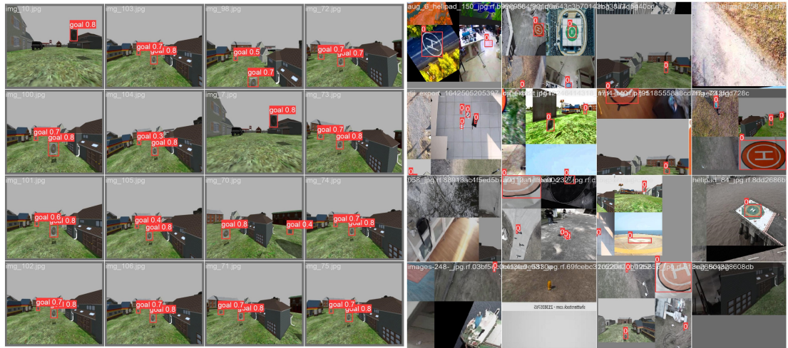
Figure 4.4: Testing results of the YOLOv8 model to detect the goal in simulated and real-world scenarios after 50 epochs
