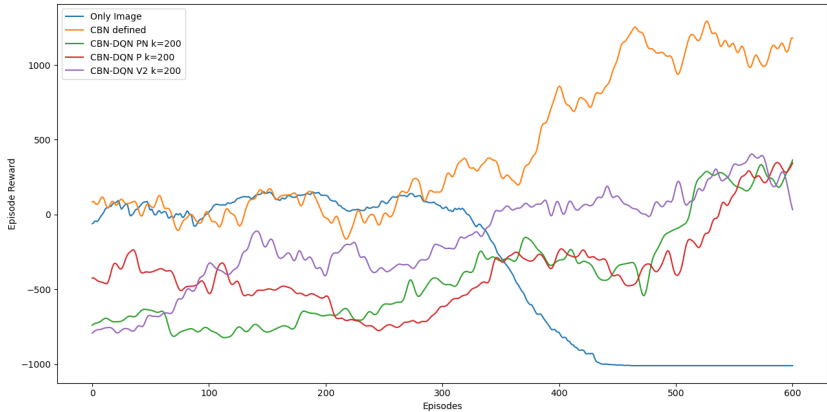
Figure 5.4: Episode reward obtained after 700 episodes with base DQN, DQN with the CBN defined, CBN-DQN PN, CBN-DQN P, and CBN-DQN V2 with k=200 , with a moving average of 50.
