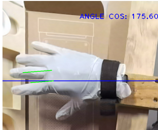
Figure 5.28: Experimental result during hand rotation, an angle of 175 degrees can be observed in this image, approximately 180 degrees, with the fingertips oriented to the left with respect to the horizontal.
