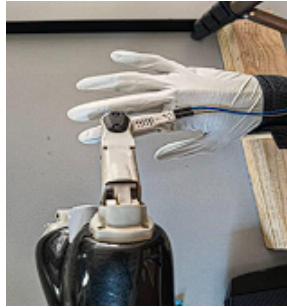
Figure 4.14: Experimental example of pressure measurement through the pressure sensor attached to the 3D hand model.
