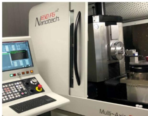
Figura 3. Fresadora CNC Moore Nanotech 650 FG multi eje [5].
