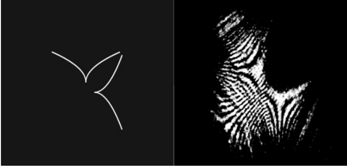
Figure 3.9: Young-cusp interferometer in two possible configurations and its corresponding interference pattern.
