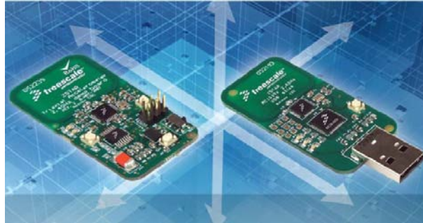
Figure 4-16 ZSTAR2 wireless kit from Freescale [14]
