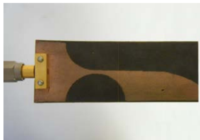
Figure 4.9. Photograph of the antipodal Vivaldi antenna used in the PMMW imaging system.
