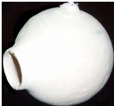
Figure 6.4. Photograph of the integrating sphere constructed by Soto et. al., [6.8].
