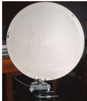
Figure 4.8. Photograph of the parabolic horn antenna used in the PMMW imaging system.
