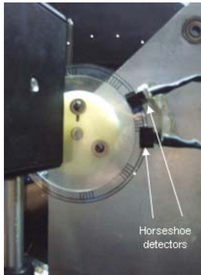
Figure 6.9. Photograph of the second disc constructed. Two horseshoe detectors are placed in the disc, one of them to inform us the beginning and end of the readings, and the other to indicate us when we have to take the reading from the photodetector and when not.
