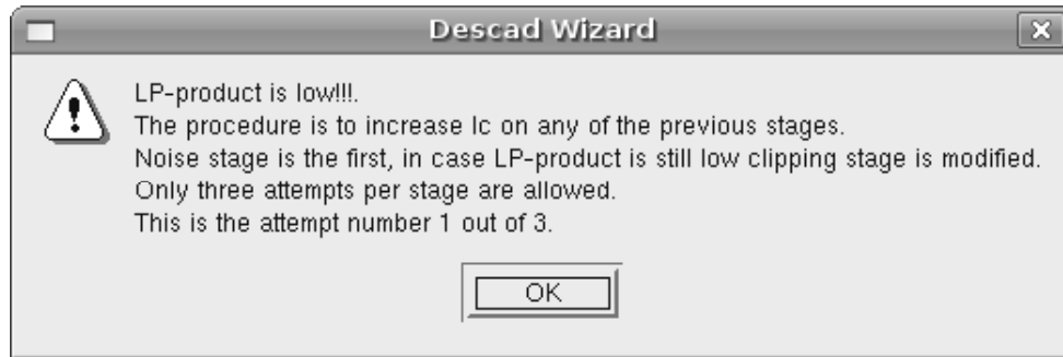
Figure 7.12: The tool informs the user that the already designed stages do not reach the desired bandwidth value.
