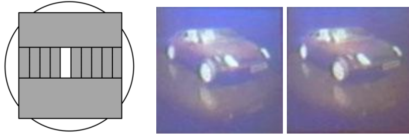
Fig. 3.5.(a)The aperture P(x_i, y_i) provides perspectives views and white light CGH in reconstruction (left), (b) 3D color image in white light playback through adjacent reconstructed aperture/windows (right)
