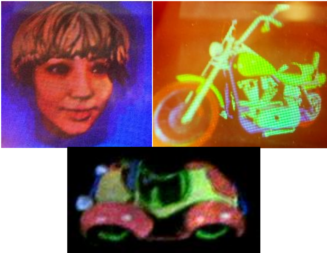
Fig. 4.12. Reflective/Lippmann parallax true-color holographic stereogram ( 4cm×4cm ), left: portrait image around hologram; right: CG bike image around hologram, below: CG car image behind of hologram. All of them are processed with imaging positioning technique and compensated the lens aberration, described above, respectively.
