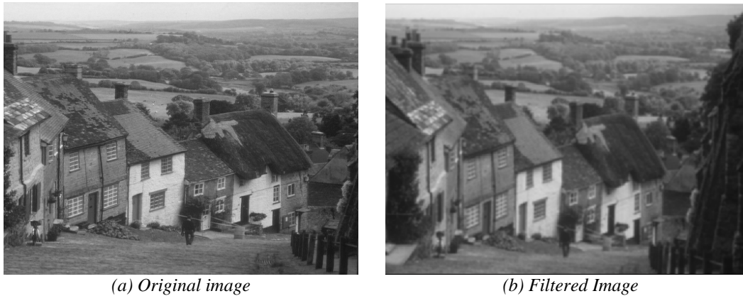
Figure 6.3 Output for convolution using Gaussian operator
