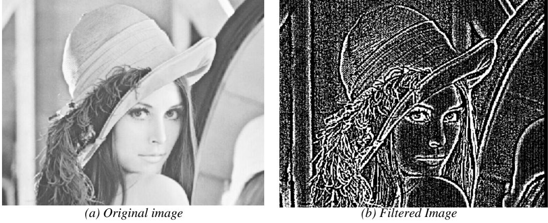
Figure 6.6 Output for high pass filter
