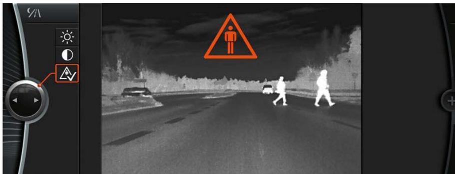
Fig. 2.2: *BMW Night Vision with pedestrian detection* [8], [9].
