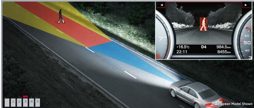
Fig. 2.1: *Night Vision with Pedestrian Detection* de AUDI [5], [6], [7].
