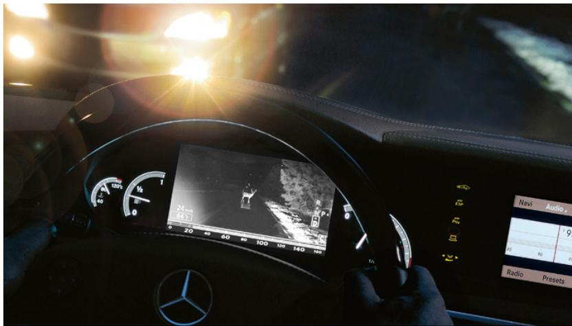
Fig. 2.3: *Night View Assist PLUS with Pedestrian Detection* de Mercedes-Benz [10], [11], [12].
