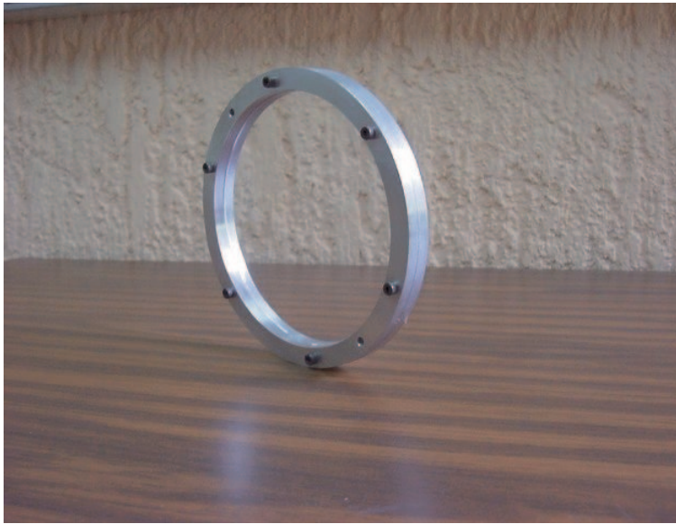
Figure 5.5: Mylar beam-splitter, held in a 140 mm diameter aluminum ring, used for the aligning process.
