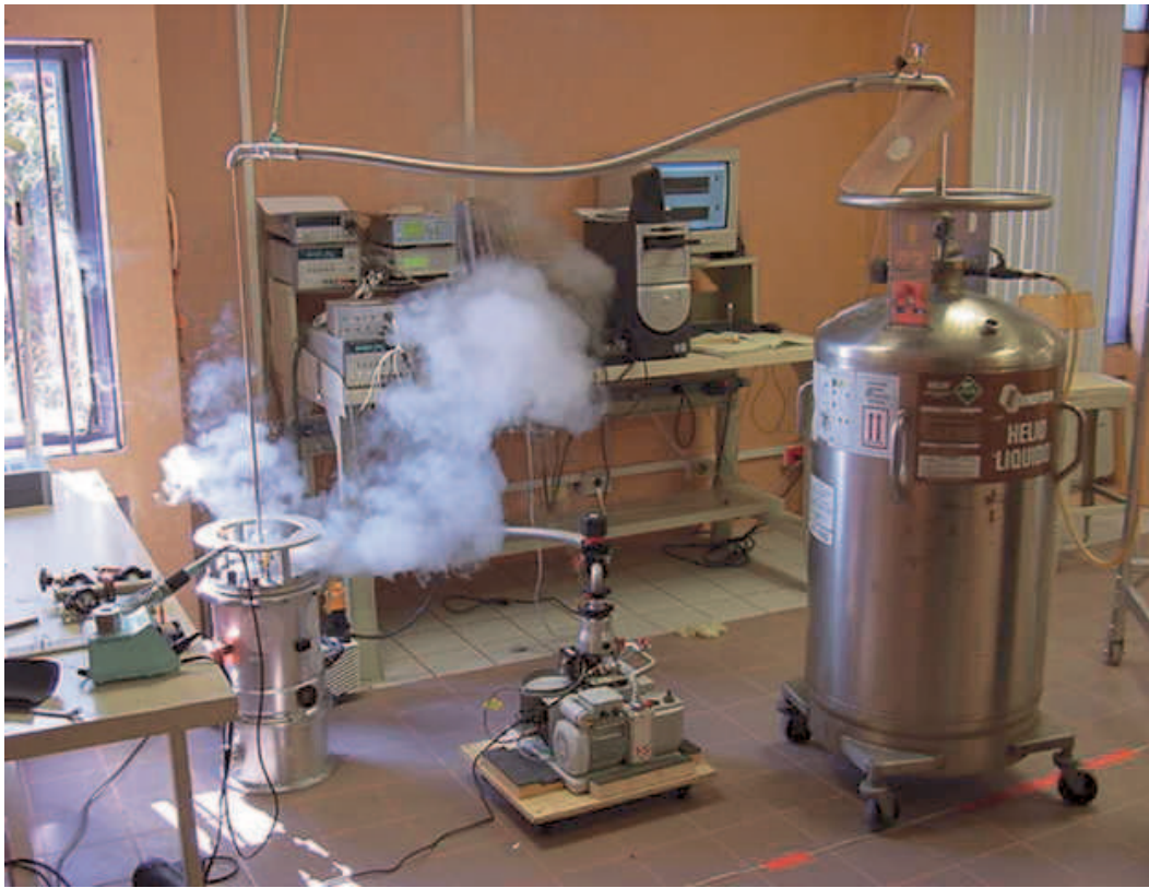
Figure 4.6: Cooling-down process during the liquid helium transfer stage.
