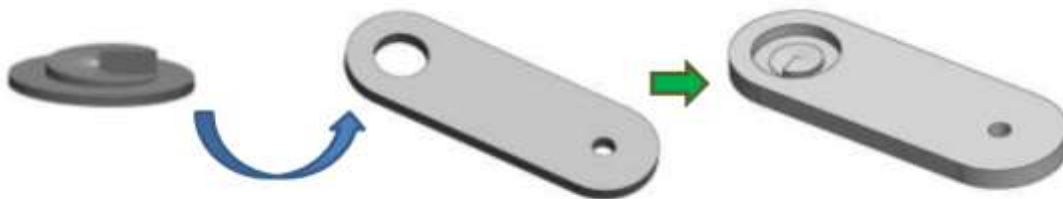
Figure 11. Diagram of the free spiral/Fixing block-guide. It is formed by two holes, the big one is for introducing the spiral as shown by the blue arrow. The small one is for holding and positioning it in the experimental set up [1].
